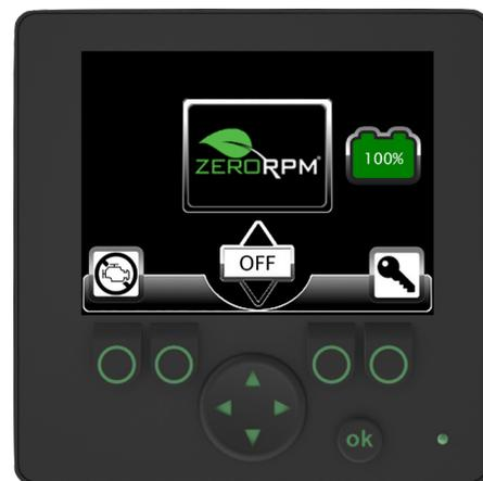
If the engine is running while the vehicle is in Park, the IMS can be engaged by holding F1. To force the engine off during idle (in Park only), press and hold F1. This will also engage ZeroIDLE Mode if applicable (see Section 8 for details).
